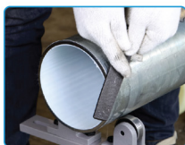
Unsharping the edges of steel pipe surfaces
