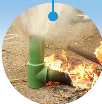
Plastic pipe are flammable and release smoke when burned, which is a major cause of fatalities in fire incidents
