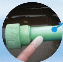
Plastic pipes become more friable and brittle after being exposure to sunlight.
